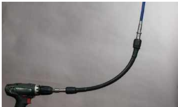
ART. 910.PR.05 - Innovative probe made with rotating shaft protected by an outer sheath that allows: - to work safely and effectively, managing to direct the rod better and to position it more centrally in the pipe to be cleaned. - insert the rod making it bend angles greater than 90 ° without straining too much the head rod.
